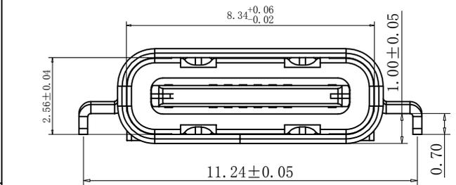
16 PIN USB Type-C Receptacle Interface (Front View)
